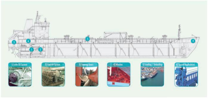
Illustration of several shipside applications for Leistritz screw pump series L2, L3, L4 and L5
