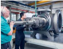
The L4NC series is equipped with a casted steel casing with integrated pump liner and a side in — top-out arrangement with ASME or DIN flanges. Leistritz has made no concession to its philosophy to manufacture spindles from one piece of metal. Thus, they realise the concept with very low shaft deflection, resulting in a long service life of bearings and shaft seals and a high efficiency.
