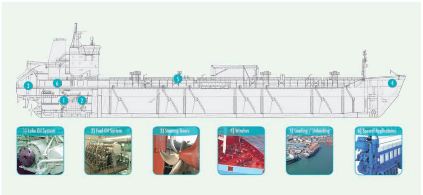
Illustration of several shipside applications for Leistriz screw pump series L2, L3, L4 and L5
