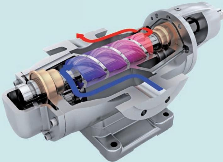
Leistriz screw pumps of the L2NG/NT series are twin screw single volute, self-priming positive displacement pumps for low pressure duty, suitable for transport of slightly abrasive and corrosive, high or low viscous fluids with poor or good lubricity.
