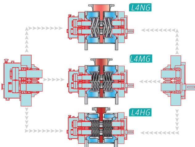
Instead of individual designs, all pumps are designed and manufactured as a modular system. While pump casings, liners and screws are still adapted to the particular operating conditions, bearing covers, bearings, timing gears and the seal components are interchangeable among pumps of different sizes.
