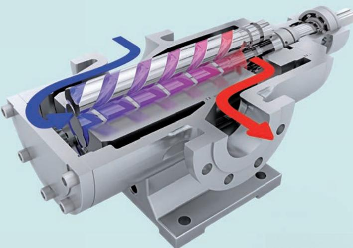
Leistriz screw pumps of the L3MG series are triple screw single volute, self-priming positive displacement pumps for medium pressure duty, suitable for transport of non abrasive, lubricating fluids.
