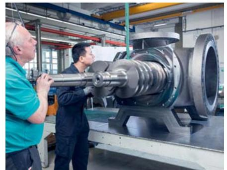
**Final assembling of spindles for L4NC**
